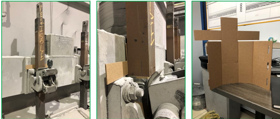
Figure 16. Anode isolation system.
